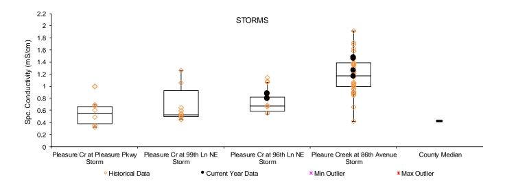
**Chlorides at Pleasure Creek.** Orange diamonds are historical data from previous years and black circles are 2019 readings. Box plots show the median (middle line), 25<sup>th</sup> and 75<sup>th</sup> percentile (ends of box), and 10<sup>th</sup> and 90<sup>th</sup> percentiles (floating outer lines).
