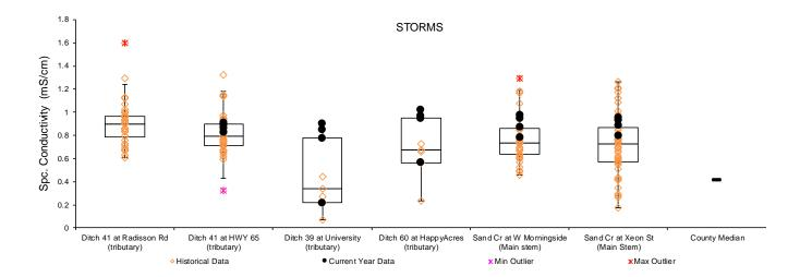
**Chlorides at Sand Creek** Orange diamonds are historical data from previous years and black circles are 2019 readings. Box plots show the median (middle line), 25<sup>th</sup> and 75<sup>th</sup> percentile (ends of box), and 10<sup>th</sup> and 90<sup>th</sup> percentiles (floating outer lines).
