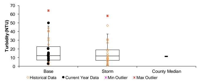
**Total suspended solids during baseflow and storm conditions** Orange diamonds are historical data from previous years and black circles are 2019 readings. Box plots show the median (middle line), 25<sup>th</sup> and 75<sup>th</sup> percentile (ends of box), and 10<sup>th</sup> and 90<sup>th</sup> percentiles (floating outer lines).
