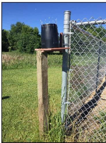
Tipping bucket rain gauge.
