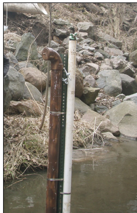
YSI EXO water quality sonde casing (white) and an OTT continuous water level monitoring device casing (brown) in Oak Glen Creek. There is a staff gage on the green post facing the other direction.
