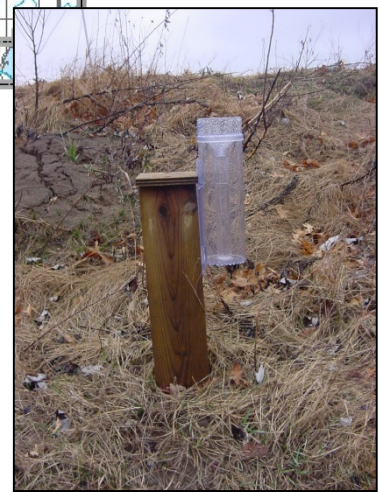
Cylinder rain gauge.
