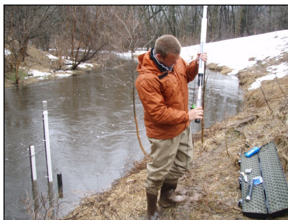
Staff deploying the Hydrolab MS5. In the background are the Hydrolab casing (shorter) and an RDS continuous water level monitoring device.
