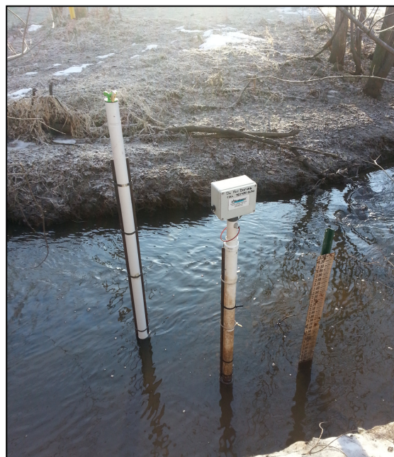
Hydrolab MS5 casing (taller) and an RDS continuous water level monitoring device at Springbrook Creek.
