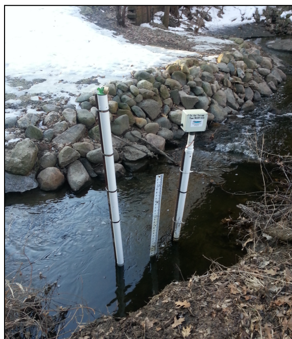
Hydrolab MS5 casing (taller) and an RDS continuous water level monitoring device in Pleasure Creek. A staff gauge is shown in the middle.
