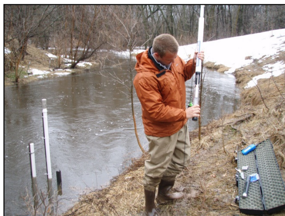
Staff deploying the Hydrolab MS5. In the background are the Hydrolab casing (shorter) and an RDS continuous water level monitoring device.
